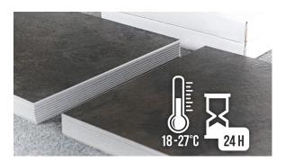
Installations in areas colder than recommended will influence the installation properties of LVT Dryback. The planks or tiles will be less flexible, cutting will be harder and small pieces difficult to cut out. The lower the temperature, the more difficult the installation. Also, the risk to have excessive expansion is increasing with decreasing installation temperature. Installation in areas warmer than recommended increases the risk for excessive shrinking/gaps between panels.
